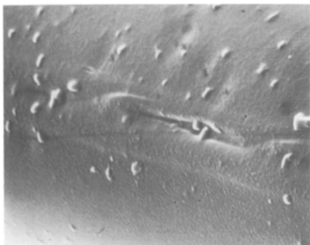
Figure 15 Surface modification revealing internal structural changes occurring during fatigue.
